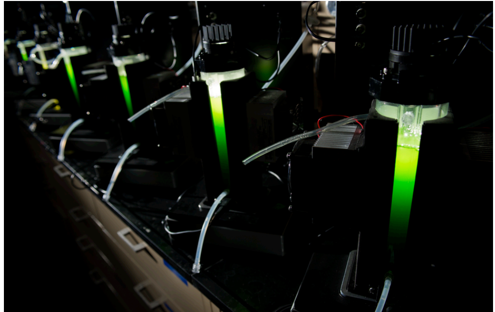
Figure 3. An ePBR matrix in action. Left panel shows a working ePBR unit and output data. The right panel is a photograph of part of a 20-unit ePBR matrix currently working in the Kramer lab.
